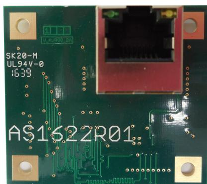
If the user wants to connect the barrier to a network in order to get a remote control, or to access the status of this network, remotely, this ETHERNET card can be added to the main control card (AS1620).
