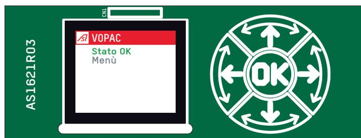
When an Ethernet network is not available, this expansion card with colour TFT display allows, via simplified menus, much more visual settings of the barrier.
