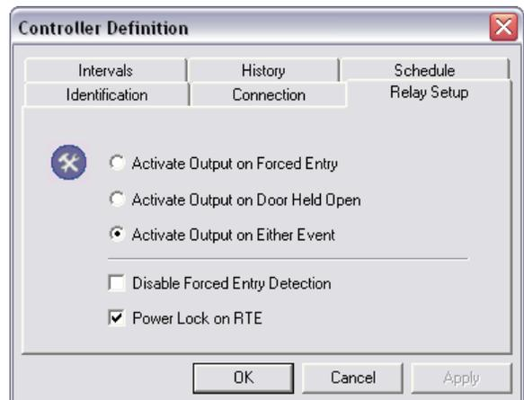
The screenshot shows the 'Controller Definition' window with the 'Relay Setup' tab selected. The 'Activate Output on Either Event' radio button is selected. The 'Disable Forced Entry Detection' checkbox is unselected, and the 'Power Lock on RTE' checkbox is selected. The 'OK', 'Cancel', and 'Apply' buttons are visible at the bottom.
