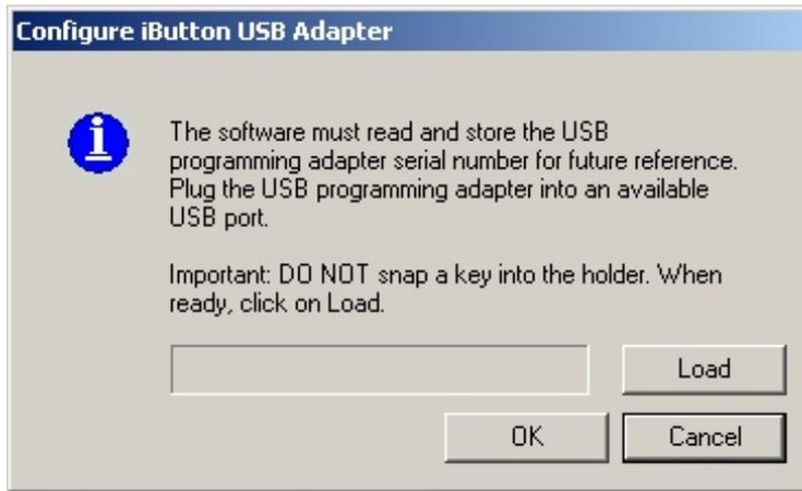
Without any iButton snapped into the holder, select **Load**.
